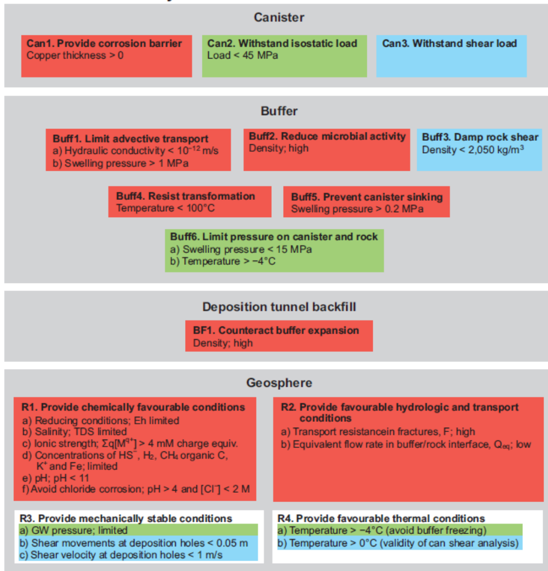
Figure 8-2. Safety functions (bold), safety function indicators and safety function indicator criteria related to containment. When quantitative criteria cannot be given, terms like “high”, “low” and “limited” are used to indicate favourable values of the safety function indicators. The colour coding shows how the functions contribute to the canister safety functions Can1 (red), Can2 (green) and Can3 (blue).
