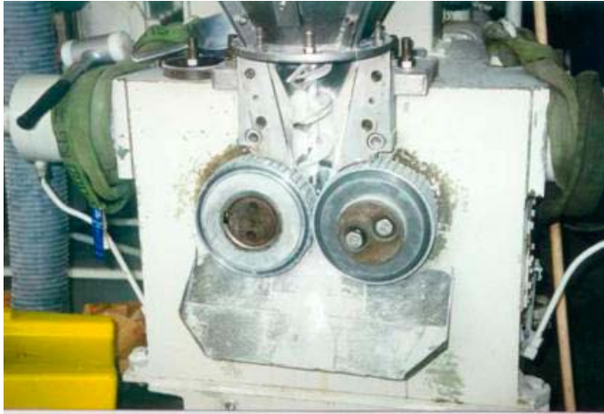
Figure 5-8. A machine for pressing of briquette shaped pellets, BEPEX test equipment.
