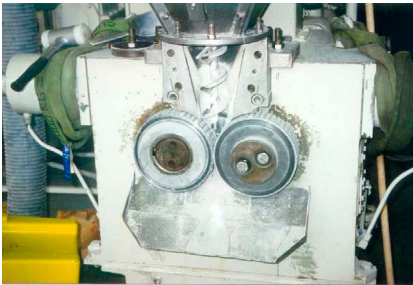
Figure 5-10. A machine for pressing of briquette shaped pellets (BEPEX test equipment).
