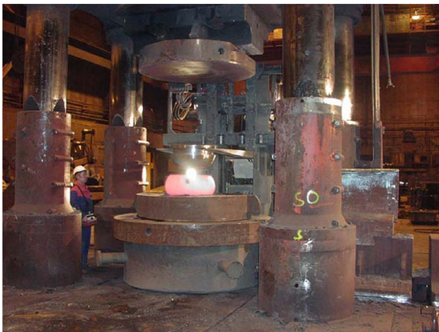
Figure 5-17. Forging of a lid blank.
