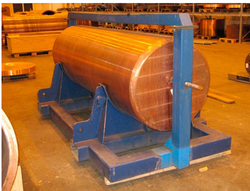
Figure 5-9. Large copper ingot weighing approximately 12 tonnes.
