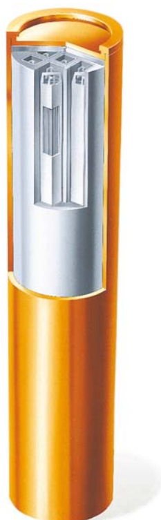
Figure 3-1. SKB's reference canister with an outer corrosion barrier of copper and an insert of nodular cast iron.
