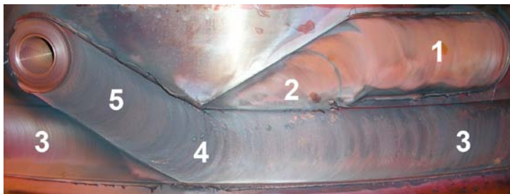
Figure 5-26. Sequences in the welding cycle: 1) acceleration sequence, 2) downward sequence, 3) joint line welding, 4) overlap sequence and 5) parking sequence.
